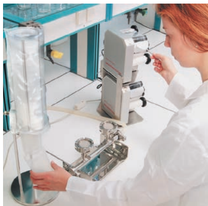
1. When taking a new presterilized funnel, the membrane is dispensed automatically
