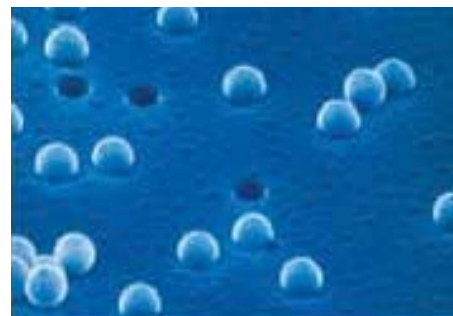
Electron micrograph of Cyclopore membrane with latex beads on surface
