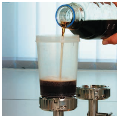
3. Liquid is poured into the funnel and a vacuum is applied
