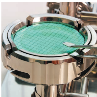
4. Membrane is easily removed after filtration
