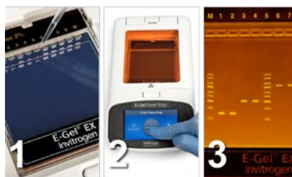
Sample analysis in three simple steps—load, run, and analyze.
