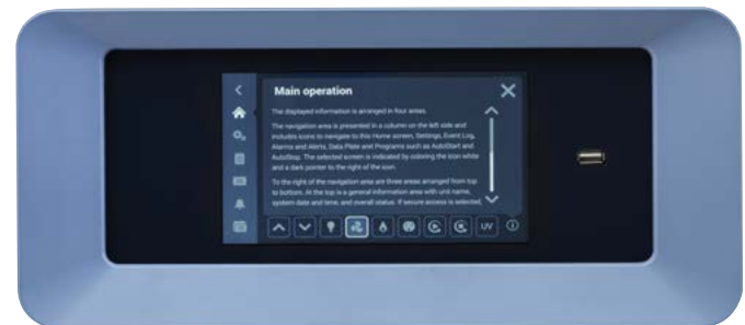
Figure 2: Herasafe 2030i BSC display in Main Operation mode
